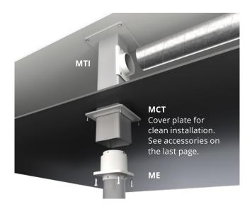
**ATEX (EX):** Aluminum and metal parts painted using special conductive paint (black), conductive polypropylene duct connection. Earth cable for safe grounding. Complies with the ATEX Directive 2014/34/EU category 2 gases and dust.
